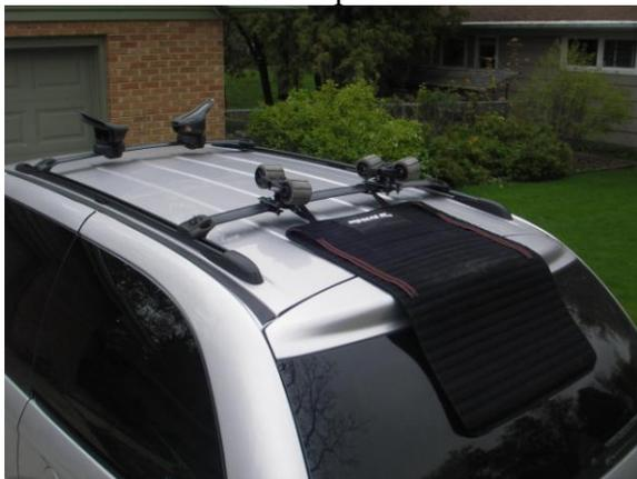
It's called a "water slide" made by Thule. It is ribbed on one side and rubber backed on the other. I added two nylon straps with Velcro at the top of the slide so it could be rolled up and held against the cross member
